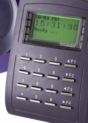
The AR-727HB-RAY is an extremely versatile controller/reader operating either as a standalone controller or as a network controller as one of up to 254 controllers operating via an RS485 connection to a host PC.
