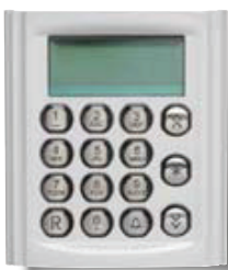
Type 8017 Control module with keypad and display for encoded door lock release and equipped with relay output for door lock release and 3 additional outputs to drive relay type 170/001. The door lock opening codes can be entered either via the keypad (100 different codes) or using keys type 89TK (500 different codes) interfaceable with modules 80TK. Module 8017 can connect up to 4 independent 80TK modules. Supplied with software for additional management of module via PC. Type 6952 is required for interfacing via PC. Requires power supply type 6582 and frame types 8D81, 8D82, 8D83, 8D84.
