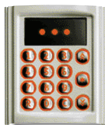
Type 8016 Control module with encoded lock, equipped with relay output for door lock release and additional output to drive relay type 170/001. Requires power supply type 6582.
