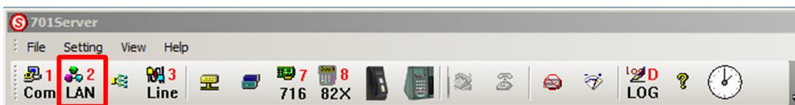
Each controller on a network must have a unique Node ID. We would recommend setting controller Node ID's from ID=2 upwards (This will enable a USB desktop reader to be used if required) Select 2 LAN as shown above from the 701 Server header strip to access Node ID setting.
