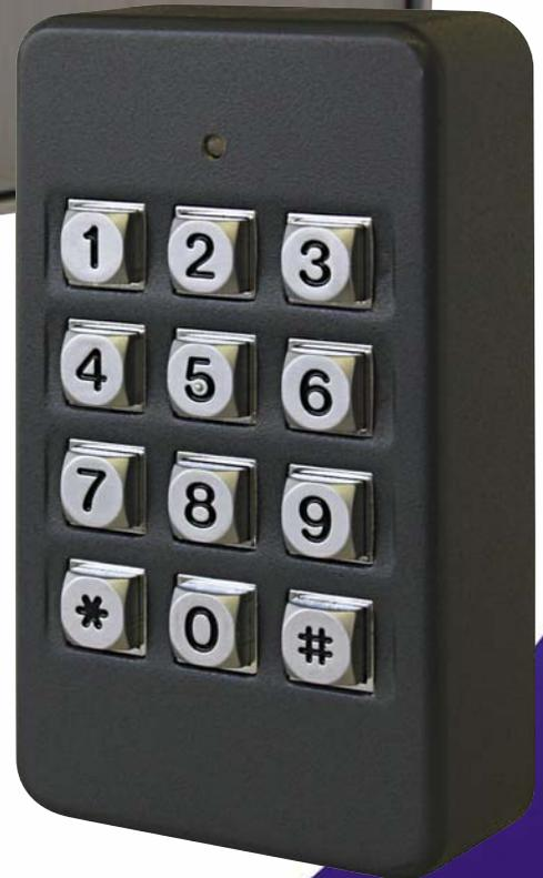
The K50i series Access Controller is a fully encapsulated controller with a robust, engraved metal keypad and either a plastic cover for surface mounting or a stainless steel vandal resistant case for surface mounting and a stainless steel front plate that fits onto a standard double gang electrical back box for flush mounting.
