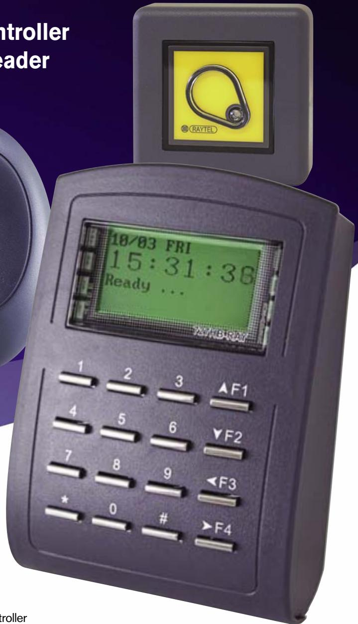
The AR-727HB-RAY is an extremely versatile controller/reader operating either as a standalone controller or as a network controller as one of up to 254 controllers operating via an RS485 connection to a host PC.
