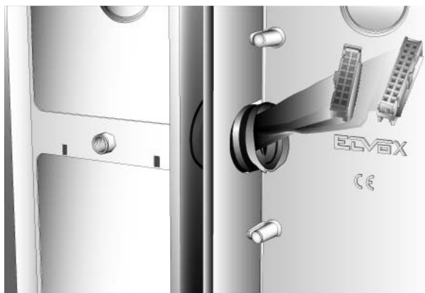
Fig. 4 - The figure shows in detail the passage of connectors and respective flat cables for the cabling of different modules through the corrugated tube.
