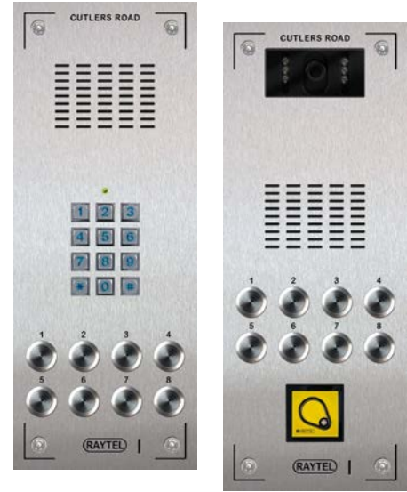
Raytel Spartan Large - Surface or Flush Mount Video and Audio Door Entry Panels available as Functional (1 to 35 apartments) or Digital Dial (1 to 6400* apartments) with optional Access Keypad or Proximity Token Reader.
